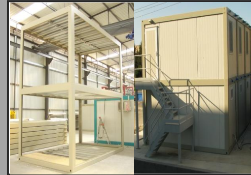
The use of a single middle chassis in multi storey structures that serves both as a floor and a ceiling
