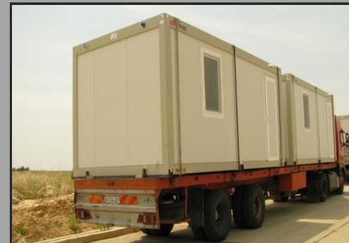
2 units of 20 feet assembled modules can be loaded in a single TIR truck
