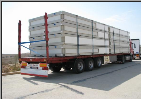
8 units of 20 feet modules can be loaded in a single TIR truck
